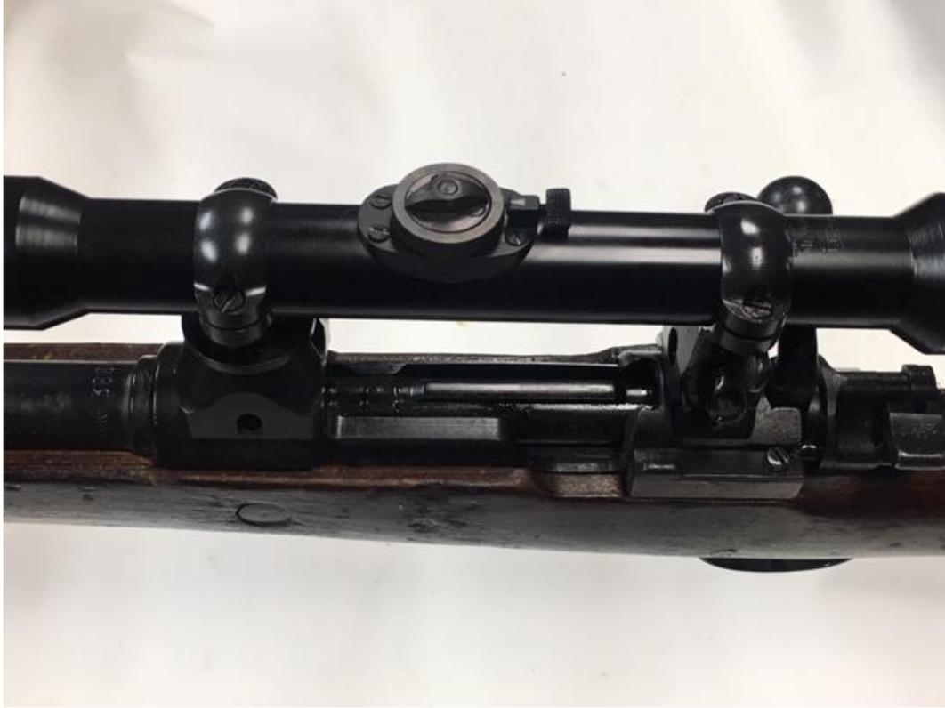
Note: Ensure that the rear locking lever is tight to lock the ring into position on the base.
